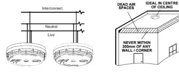
Be very careful about correctly wiring the alarms as mixing Live and Neutral will blow/damage interconnected alarms.
