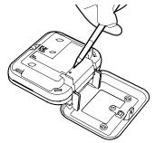
Using a ballpoint pen, briefly push and release the 'learn button' on the back of Alarm 2. The red LED next to the learn button will flash briefly then light up for approximately five seconds.
